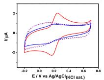
formed by the template molecules. The voltammograms obtained using NIP-cortisol and MIP-cortisol modified electrodes shown almost the same voltammetric behavior obtained for NIP modified electrode due to the difficult of the redox probe to achieve the electrode surface demonstratting a great potential for selective recognition of cortisol suing a MIP modified electrode.
