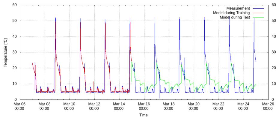
**Figure 1** - Model of the temperature inside the milk tank based on input data  $x_1$ ,  $x_2$ , and  $x_3$  during an excerpt of the training horizon (red) and the testing horizon (green) plotted against the actual measurement (blue).
