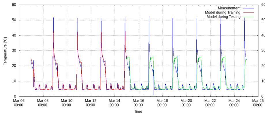
**Figure 2** - Model of the temperature inside the milk tank based on input data  $x_1, \dots, x_8$  during an excerpt of the training horizon (red) and the testing horizon (green) plotted against the actual measurement (blue).
